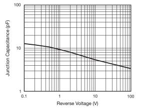
Fig. 6 - Typical Junction Capacitance
