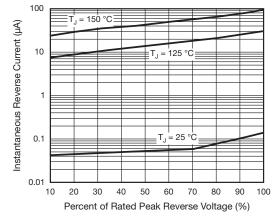
Fig. 5 - Typical Reverse Leakage Characteristics
