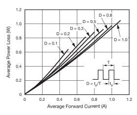
Fig. 2 - Forward Power Loss Characteristics
